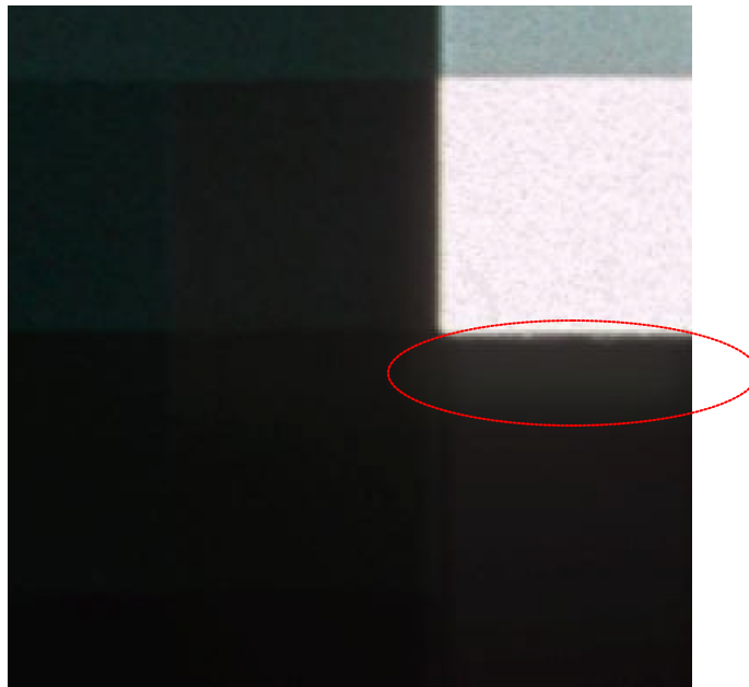
Figure 7: A typical ghosting effect along a high contrast edge. The area circled in red is lighter than normal due to the flare defect. This type of defect reduces image quality and can significantly compromise the accuracy of custom scanner profiles.
